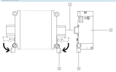
The valve terminal is attached to the H-rail and locked with the swivel lever.
