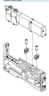
The fixed restrictor can be used to permanently set the flow rate when venting in ducts 3 and 5.
