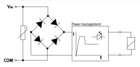
Each solenoid coil is protected with a spark arresting protective circuit as well as against polarity reversal.
