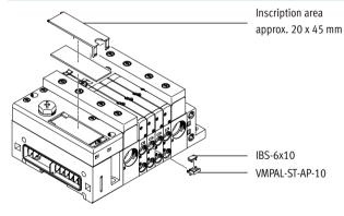
A holder VMPAL-ST-AP-10 (Part No. 561109) with inscription labels (Part No. 18576, IBS-6x10) can be mounted on each sub-base for labelling the valves.
