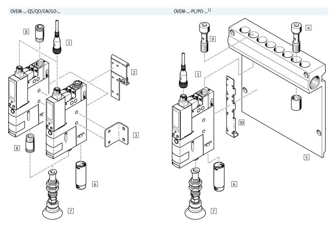
1) Hollow bolt 2) and mounting bracket 10 are included in the scope of delivery of the OVEM-...-PL/PO-....
