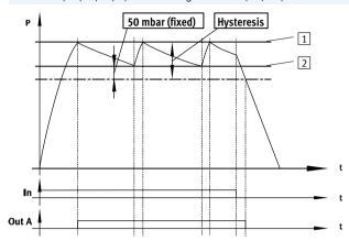
If the desired threshold value 1 for the vacuum is reached, vacuum generation is automatically switched off. A non-return valve prevents the reduction of the vacuum. Nonetheless, leakage (e.g. due to rough workpiece surfaces) will
