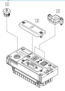
Covers are inserted/screwed into or placed/screwed onto unused connections/openings.
