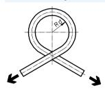
The tube is bent in the direction of its own curve until the tubing outer diameter is flattened by 5%. Rd is then calculated mathematically. The flow rate is not reduced until Rd is reached.
