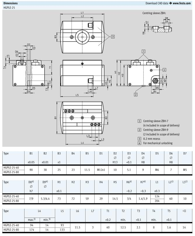
Tolerance for centring hole ±0.02 mm Tolerance for thread ±0.1 mm
