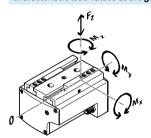
The indicated permissible forces and torques apply to a single gripper jaw. They include the lever arm, additional applied loads due to the workpiece or external gripper fingers and acceleration forces occurring during movement.
