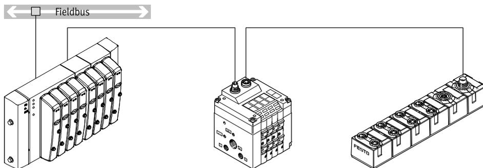
CDVI-DN valve terminals with fieldbus interfaces can be equipped with 4 to 16 valve positions at maximum 24 solenoid coils.
