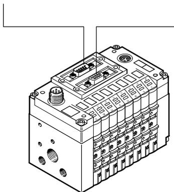
The bus connection is established via a 9-pin Sub-D socket and a 9-pin Sub-D plug with a typical INTERBUS pin allocation.
