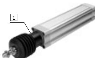
The protective bellows kit is a leak-free system. To prevent unwanted media from being drawn in, the supply and exhaust air must be ducted via a pressure compensation hole in the connection part [1].
