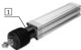
The bellows kit is a leak-free system. To prevent unwanted media from being drawn in, the supply and exhaust air must be ducted via a pressure compensation hole in the connection part 1.
