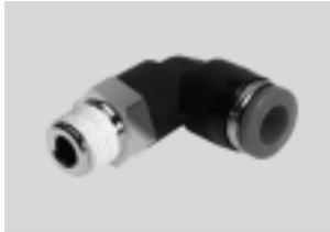
Wide selection of push-in fittings for pneumatic applications with a temperature range up to 80 °C and a pressure range up to 14 bar. Tubing O.D.∅ of 4, 6, 8, 10, 12 and 16 mm with connecting threads R1/8 ... R1/2 and G1/8 ... G1/2.
