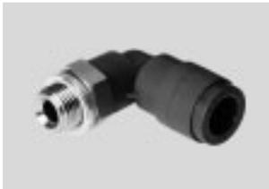
Flame-retardant push-in fitting for use in all areas where there is a risk of fire, for example welding systems in the automotive industry and in the construction industry. For pneumatic applications with a temperature range up to 60 °C and a pressure range up to 10 bar. Tubing O.D.∅ of 4, 6, 8, 10 and 12 mm with connecting threads R1/8 ... R1/2 and G1/8 ... G1/2.
