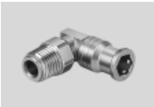
Stainless steel push-in fitting. High corrosion resistance (CRC4) and chemical resistance with approval for use in the food and packaging industry. For pneumatic applications with a temperature range up to 120 °C and a pressure range up to 10 bar. Tubing O.D.∅ of 4, 6, 8, 10, 12 and 16 mm with connecting threads M5 and R1/8 ... R1/2.
