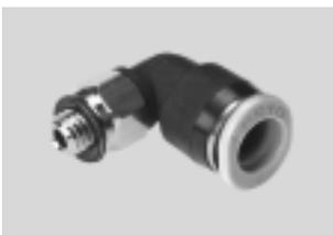
Miniature push-in fittings for maximum component density in confined spaces. For core pneumatic applications with a temperature range up to 60 °C and a pressure range up to 10 bar. Tubing O.D.∅ of 3, 4 and 6 mm with connecting threads M3, M5, M7 and R1/8.
