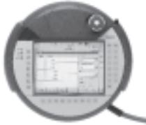
When creating a motion program, the motion sequence is very often known but the precise position to be approached, for example of a gripper or a tray is not. These can only be determined directly during commissioning by means of accurate approaching. The CMXR in combination with the teach pendant CDSA offers dialogue-based software for this purpose, thus enabling quick and easy teach-in of the necessary positions.
