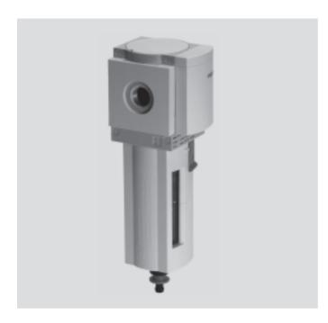
Active carbon filters remove liquid and gaseous oil particles as well as odor and taste from compressed air. Pre-filtration with a grade of 0.01 micron is required.
