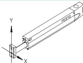
As long as the centre of gravity of the effective load on the yoke plate lies within the outline of this plate, it is impossible to overload the linear module.
