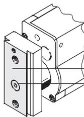
When dovetail mounting components are used, the centre of gravity should be within this area.
