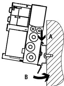
The valve terminal VTUG is attached to the H-rail (see arrow A).
