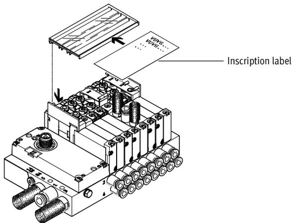
An inscription label holder ASCF-H-L1 (code TT) can be mounted for labelling the valves. The inscription label holder can be opened for inserting the inscription label and for actuating the manual override. The inscription label holders are available in different sizes depending on the number of valves.
