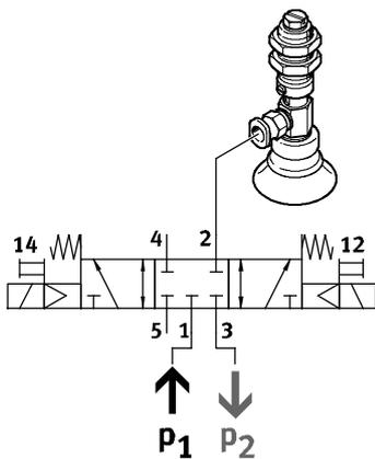
Vacuum, ejector pulse and normal position with internal pilot air can be achieved by connecting vacuum
