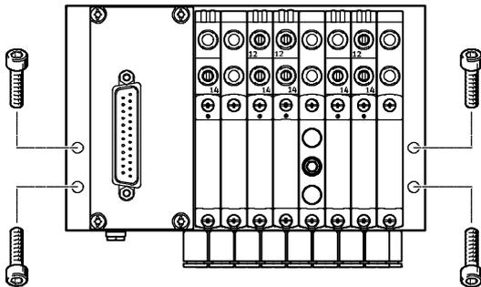
The valve terminal VTUG is screwed onto the mounting surface using four M4 screws.
