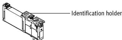
The identification holder ASLR-D-L1 (code TV) can alternatively be used to label the individual valves. This identification holder is placed directly on the manual override.
