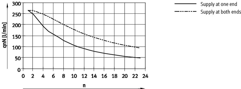
Standard flow rate  $q_n$  as a function of the number of switched valves  $n$ , size 14
