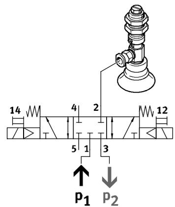
Vacuum, ejector pulse and normal position with internal pilot air can be achieved by connecting vacuum
