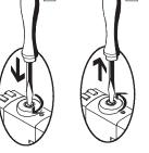
1 Press in the stem of the MO with a pin or screwdriver until the valve switches and then turn the stem clockwise by 90° until the stop is reached.
