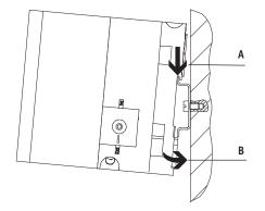
The MPA-F valve terminal is attached to the H-rail (see arrow A). The valve terminal MPA-F is then swivelled onto the H-rail and secured in place with the clamping components (see arrow B). For H-rail mounting of the valve terminal you will need the following MPA-F mounting kit:
