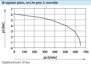
Supply pressure 10 bar, set regulator pressure 6 bar
