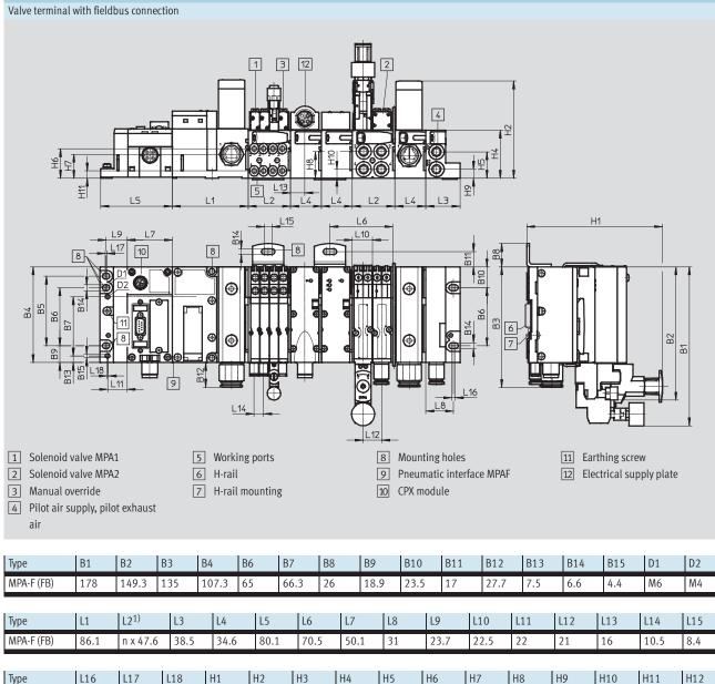
109 1) n = number of sub-bases (with MPA1, width 10 mm, max. 4 valve positions on sub-base; with MPA2, width 20 mm, max. 2 valve positions on sub-base)
