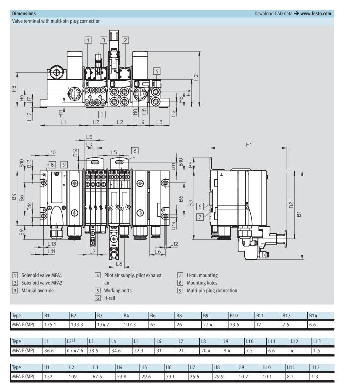
1) n = number of sub-bases (with MPA1, width 10 mm, max. 4 valve positions on sub-base; with MPA2, width 20 mm, max. 2 valve positions on sub-base)
