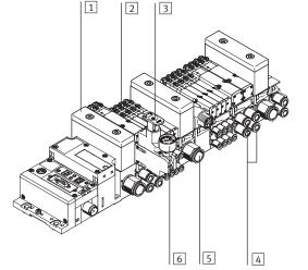
Electrical connection and display components for fieldbus
