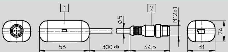
The technical drawing shows a side view of the adapter with the following dimensions: a total length of 300 ±10 mm, a USB Mini B connector section of 56 mm, a central shaft with a diameter of  $\phi 5$  mm, and an M12x1 male connector section of 44.5 mm. The M12 connector has a height of 24 mm and a width of 31 mm. Callout 1 points to the USB Mini B connector, and callout 2 points to the M12x1 male connector.
