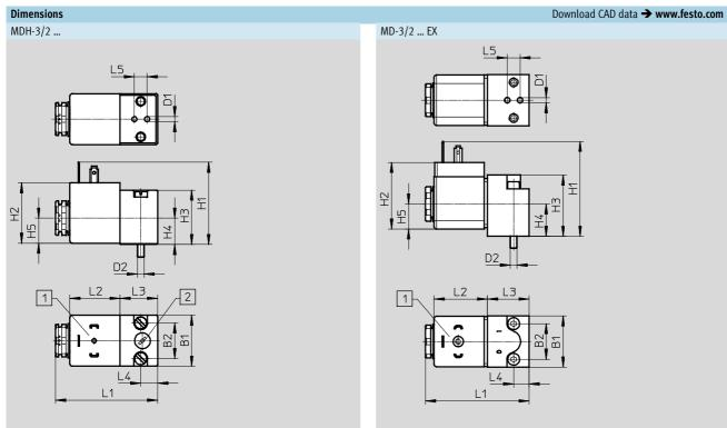
Connection dimensions and device plug to EN 175301-803, type A
