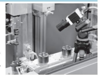
Stationary mounting of the high-speed camera to increase the availability of automation systems
