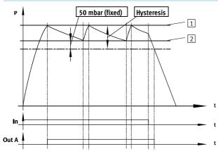
If the desired threshold value 1 for the vacuum is reached, vacuum generation is automatically switched off. A non-return valve prevents the reduction of the vacuum. Nonetheless, leakage (e.g. due to rough workpiece surfaces) will slowly reduce the vacuum. If the pressure drops below the threshold value 2, vacuum generation is automatically switched on. Vacuum is generated until the set threshold value 1 is reached again.
