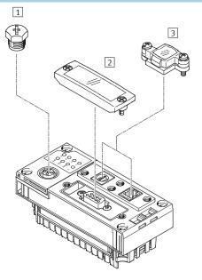
Covers are inserted/screwed into or placed/screwed onto unused connections/openings.
