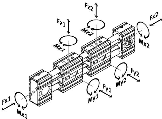
If the axis is subjected to more than two of the indicated forces and torques simultaneously, the following equation must be satisfied in addition to the indicated maximum loads:
