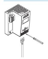
The AS-interface network as well as the power supply for the gateway and AS-interface are connected via a terminal strip.
