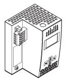
AS-interface gateways are used to connect the AS-interface network to a higher-level fieldbus.
