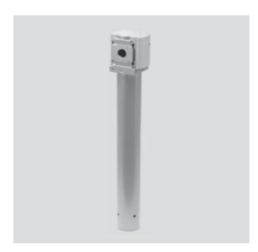
Membrane air dryers remove water vapor from the compressed air and lower the dew point preventing moisture from forming downstream. Pre-filtration with a grade of 0.01 micron is required.
