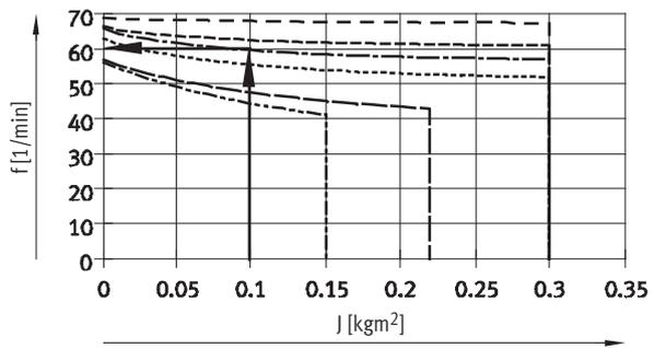
$$T_{\text{mín.adm.ciclo}} = \frac{60\text{s}}{59} = 1,017\text{s} = 1017\text{ms}$$
