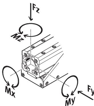
If the cantilever axis is simultaneously subjected to several of the forces and torques listed below, the following equation must be satisfied in addition to the indicated maximum loads:
