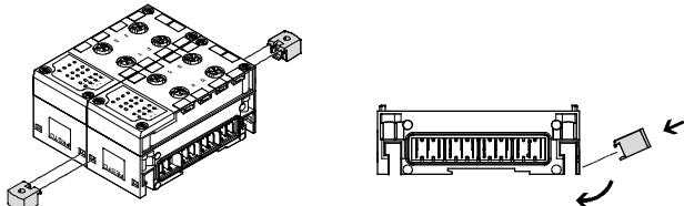
Additional mountings for the CPX terminal that can be fitted between two modules are available for longer valve terminals.
