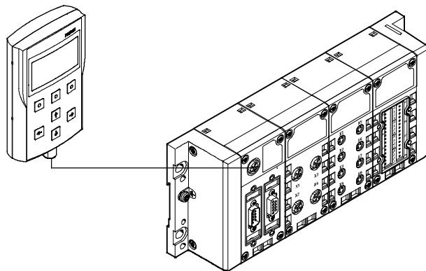
The operator unit is connected to the CPX terminal using pre-assembled cables.
