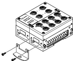
Additional mounting brackets for the CPX terminal that can be screwed onto the interlinking blocks are available for longer valve terminals.
