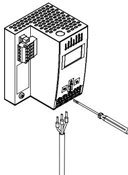
The AS-interface network as well as the power supply for the gateway and AS-interface are connected via a terminal strip.
