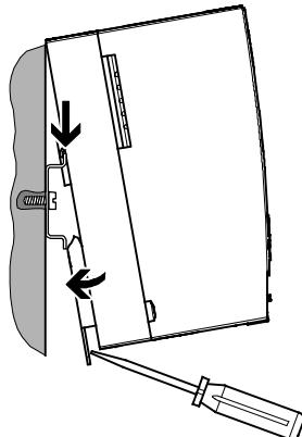
The gateway is mounted using an H-rail. There are appropriate lugs on the rear of the device.
