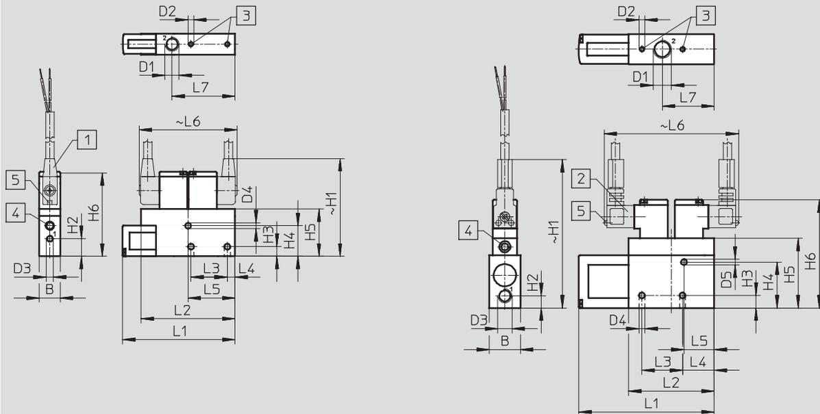
1 Socket type KMYZ-2-24-... with 2-wire cable, 2.5 or 5 m long,  $\varnothing$  3.4 mm (2x 0.25 mm<sup>2</sup>)
