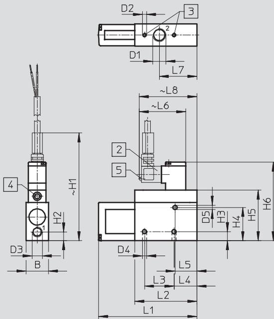
1 Socket type KMYZ-2-24-... with 2-wire cable, 2.5 or 5 m long,  $\varnothing$  3.4 mm (2x 0.25 mm<sup>2</sup>)
