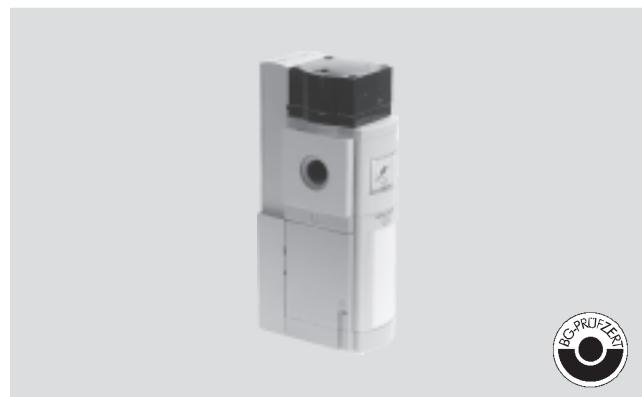
The electropneumatic soft-start and exhaust valve is used to reduce pressure quickly and reliably and to build up pressure gradually in industrial pneumatic systems and terminals. The device is a self-testing, redundant mechatronic system conforming to the requirements of EN ISO 13849-1. The
