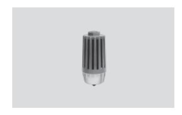
The filter silencer cleans all exhaust air from pneumatic control systems. The exhaust air is discharged into the atmosphere via a fine filter cartridge (degree of filtration: >99.99%).
