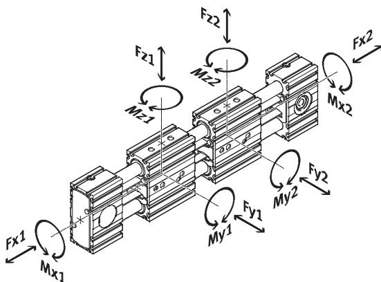
If the axis is subjected to more than two of the indicated forces and torques simultaneously, the following
