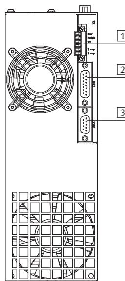
[1] Control connection for relay driver supply
