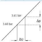
The response sensitivity of the device determines how sensitively one can change, i.e. adjust, a pressure. The smallest setpoint value difference that results in a change in the output pressure is referred to as the response sensitivity. In this case, 0.01 bar.
