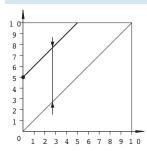
If, for example, a VPPM cannot be vented for safety reasons, the minimum pressure can be increased from the zero point. The smallest setpoint value is then assigned an output pressure of 5 bar, for example, and the largest setpoint value an output pressure of 10 bar. Zero suppression is automatically switched off if zero offsetting is used.
