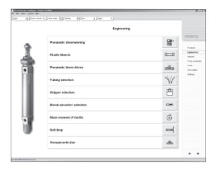
No matter whether you have discs, blocks, push-on flanges, grippers, etc: This tool does the job of calculating all mass moments of inertia for
