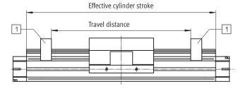
1 Fixed stops, mounted on drive or externally
