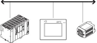
All parameters can be modified and all inspection results and characteristic values can be read via the process interface with EasyIP and Telnet.
