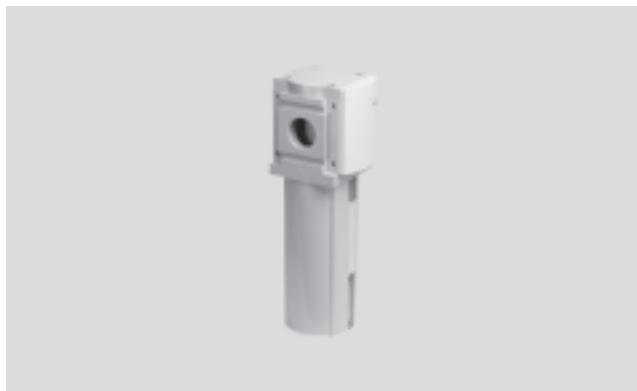
The sintered filter with centrifugal separation removes contamination, rust and condensate from the compressed air. The filter cartridges are replaceable.
