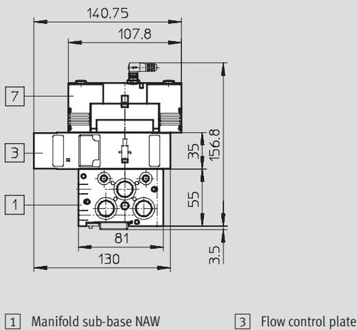
With manifold sub-base and solenoid valve (plug type C)
