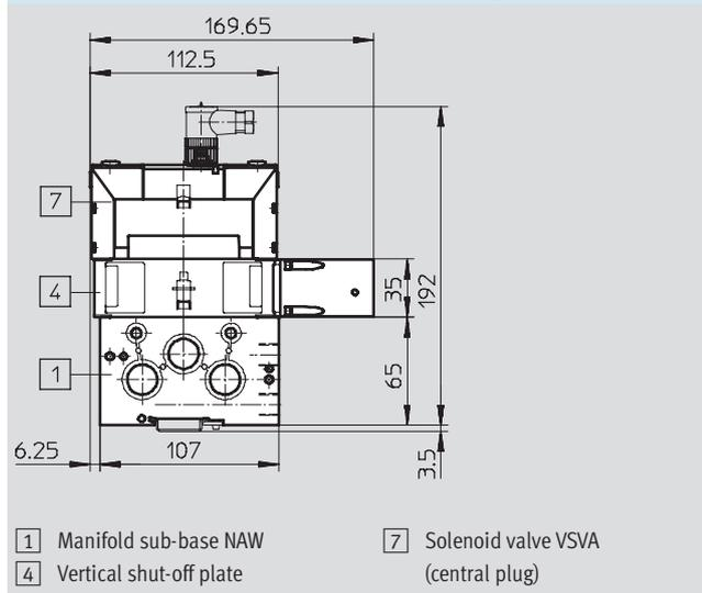
With manifold sub-base and solenoid valve (plug type C)
