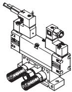
The directional control valve has a pilot control to ISO 15218 and a plug pattern to DIN EN 175301-803, type C.
