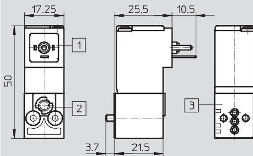
1 Connection dimensions and device plug to DIN EN 175301-803, type C
