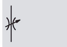
Flow control acting at both sides GRLO
