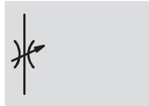
Flow control acting at both sides GRLO
