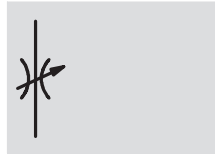
Flow control acting at both sides GRLO
