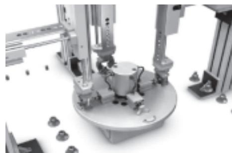
Rotary table with stationary centre section
