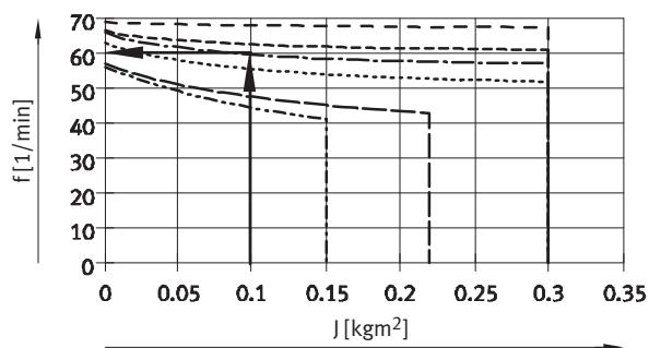
$$T_{\text{min. perm. cycle time}} = \frac{60\text{s}}{59} = 1.017\text{s} = 1017\text{ms}$$
