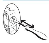
Manual override is actuated by pushing it with a pointed object or screwdriver and reset by spring force.
