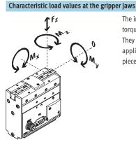
The indicated permissible forces and torques refer to a single gripper jaw. They include the lever arm, additional applied loads caused by the workpiece or external gripper fingers, as
