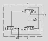
Festo "Soft-start" valves are designed to provide slow pressure build-up in pneumatic systems preventing sudden, high pressure air surges during start-up. Manual override is built in.
