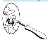
Manual override remains active until it is reset with a screwdriver.
