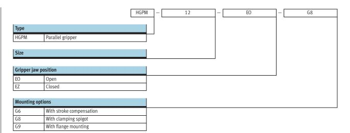
Function Single-acting with open gripper jaws HGPM-...-EO-G...
