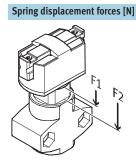
Theoretical actuating force due to stroke compensation for design variant with stroke compensation.
