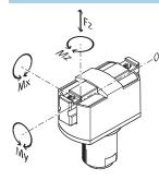
The indicated permissible forces and torques apply to a single gripper jaw. The indicated values include the lever arm, additional applied loads caused
