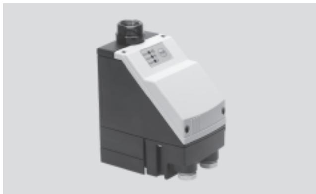
Condensate passes through the port in the bottom of the filter bowl into the attached condensate drain valve, where it is collected in a reservoir. A capacitive sensor detects once the maximum filling level is reached. The condensate escapes into the atmos-
