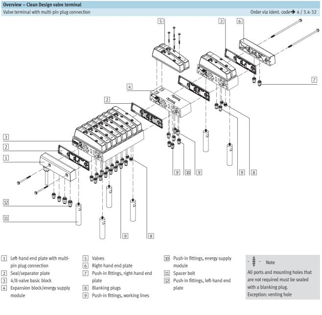
The collected exhaust air from the pilot solenoid coils of the valves is drawn off via the pressure relieving hole (venting hole) on the rear side. If you have included fittings with your order, the pressure relieving hole is also equipped with a QS fitting.
