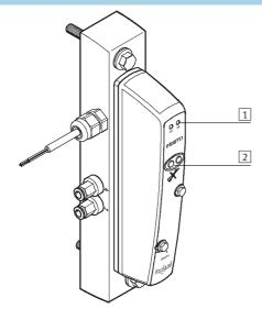
solenoid)≁ 2 Non-detenting manual override (one per solenoid valve coil)
