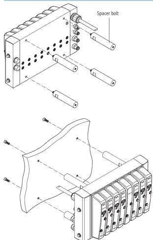
The CDVI can be mounted directly on earthed mounting surfaces using the four threaded holes in the basic block and the spacer bolts ordered via the order code (accessories order code Y).
