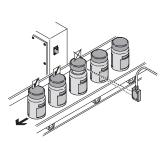
• The laser beam of a retro-reflective sensor SOEL-RSP can thus be set to detect variations in alignment.
