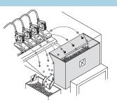
• Parts are sorted by colour using the colour sensor SOEC-RT-Q50.
