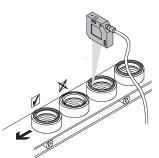
• Detection of O-rings using the laser sensor SOEL-RTH with background suppression.
