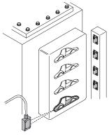
• After moulding, the laser retro-reflective sensor SOEL-RSP detects whether the workpieces are still in the metallic mould.
