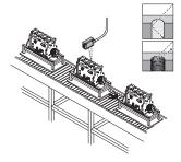
• The laser contrast sensor SOEL-RT-Q20 can detect a thread, even in a hole.
