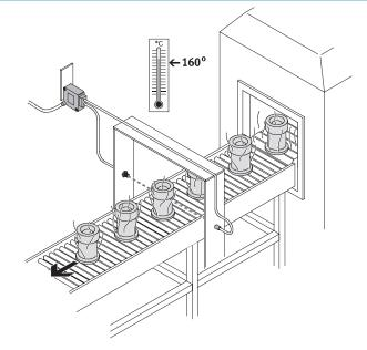
• SOEG-L can be combined with SOEZ-LLG glass fibre-optic cables to detect objects in high-temperature environments.
