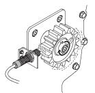
• Proximity sensing of the teeth of a gearwheel for monitoring of the machine speed
