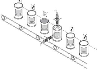
• Detection of cans and checking for the presence of the lid
