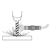
• Monitoring tools (drill breakage)
