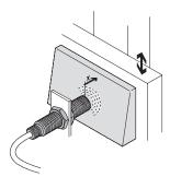
Conversion of linear motion into an electrical signal using a wedgeshaped conduction component.
