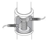
• Detection of valve positions
