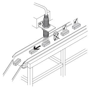
Monitoring of metallic workpieces for position, size or material, for example.
