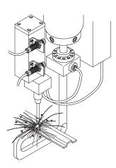
• It can also be used directly next to welding electrodes.
