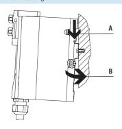
The VTSA/VTSA-F valve terminal is attached to the H-rail (see arrow A). It is then swivelled on the H-rail and secured in place with the clamping component (see arrow B).
