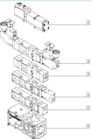
The following component sequence is recommended for valve positions with vertical stacking:
