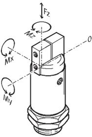
The indicated permissible forces and torques apply to a single gripper jaw. Static forces and torques relate to additional applied loads caused by
