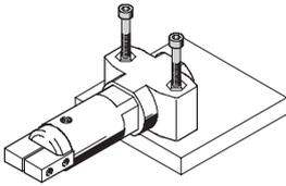
With through-holes, screws and retaining nuts
