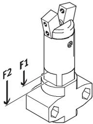
Theoretical actuating force due to stroke compensation for design variant with stroke compensation.
