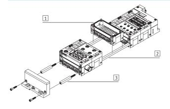
The mechanical connection between the CPX modules is created using special tie rods 2. Two screws in the end plates are all that are needed to assemble the entire unit.
