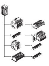
The CPX-CP electrical interface establishes the connection to CP modules of the CPI installation system via prefabricated cables. The I/O data of the connected valve terminals with CP string extension and CP input and output modules is transferred to the connected CPX bus node and thus via fieldbus to the higher-order controller. This permits the realisation of modular centralised and compact decentralised concepts with one system.
