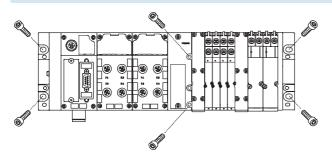
The end plates of the CPX terminal, the valve terminal and the pneumatic interface include mounting holes for wall mounting.
