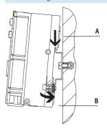
The H-rail mounting is formed in the reverse profile of the CPX interlinking blocks. The CPX terminal can be attached to the H-rail using the H-rail mounting.
