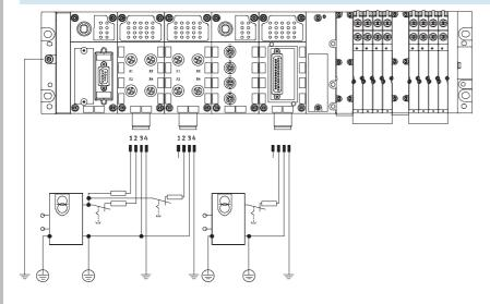
The use of decentralised devices on the fieldbus – particularly with high protection for direct machine mounting – demands a flexible power supply concept. A valve terminal with CPX can supply all voltages using a single socket.
