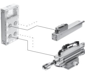
Support for the M12 connection block (8-pin) means that up to 4 cylinder-valve combinations with integrated sensors can be connected. 2 inputs and 2 outputs per socket are supported for each cylinder-valve combination. It is therefore possible to control max. 2 solenoid coils and operate 2 sensors with a pre-assembled cable.
